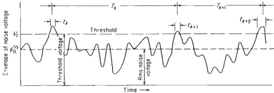
Figure.11 Envelope of receiver output illustrating false alarms due to noise.
