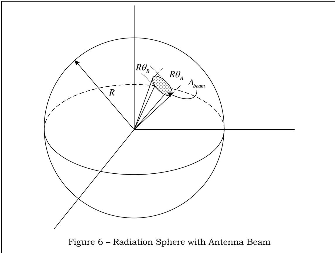
Figure 6 – Radiation Sphere with Antenna Beam
