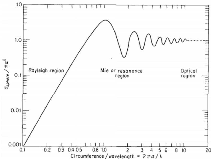
Figure 12 Radar cross section of the sphere.  $a$  = radius;  $\lambda$  = wavelength
