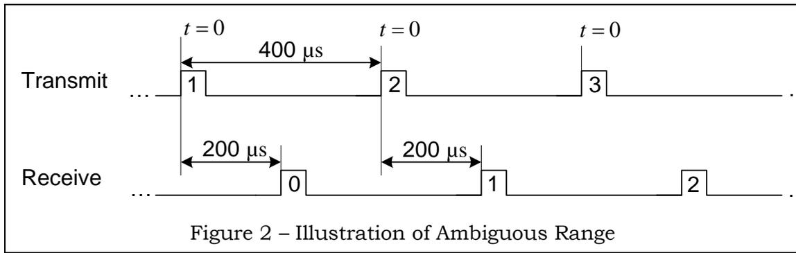
If the spacing between pulses is  $\tau_{PRI}$  we say that the radar has an *unambiguous range* of
