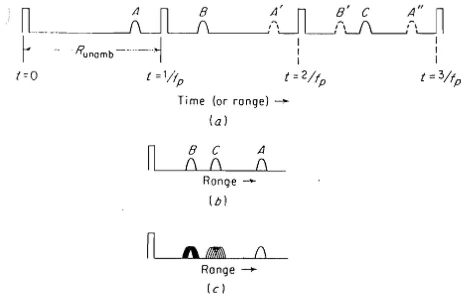
Figure.13 Multiple-time-around echoes that give rise to ambiguities in range
