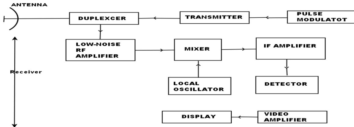
Figure 8. The block Diagram of Basic Pulse Radar System
