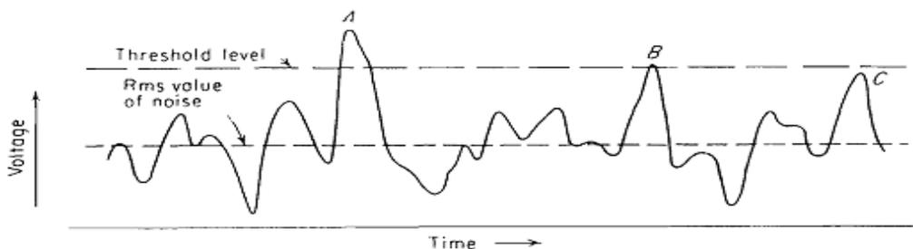
Figure.9 Envelope of radar receiver output as a function of time
