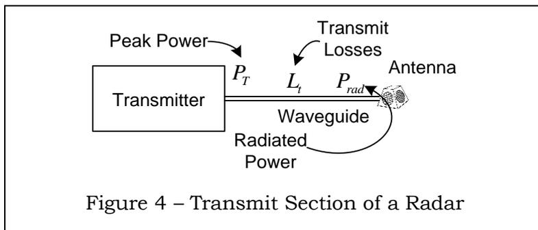
Figure 4 – Transmit Section of a Radar
