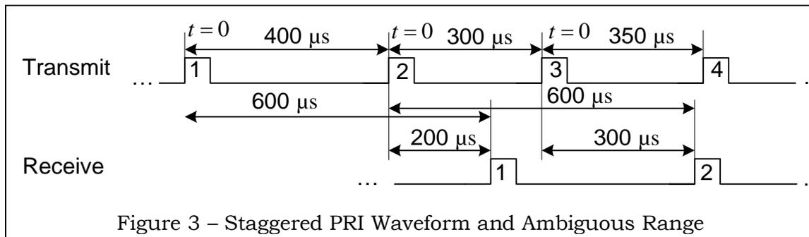
As an alternative, we could use the measured range delays in a *range resolve* algorithm to compute the true target range. Such an approach is used in pulsed Doppler radars because the PRIs used in these radars almost always result in ambiguous range operation.
