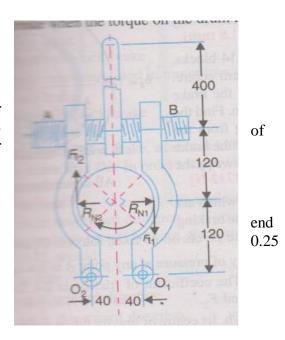
find the maximum braking torque of the drum.
